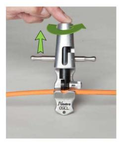
5. Install the tool on the cable with the blade located at the end of the longitudinal cut and rotate the tool around the cable to cut the jacket
