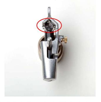
2. Set the tool in longitudinal cutting mode using D (pull + turn)
