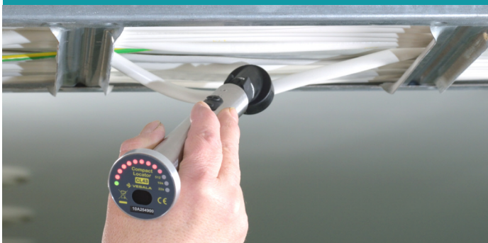
Trace and identify cables on shelves or inside structures using the close range probe
