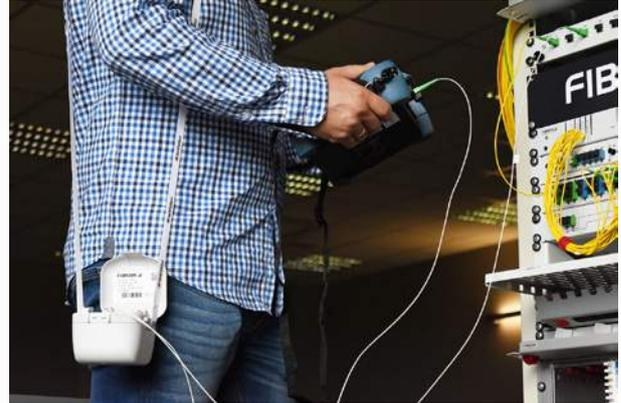
**Pic 6.** Shoulder strap facilitates the movement of the FIBRAIN OSC starter cube
